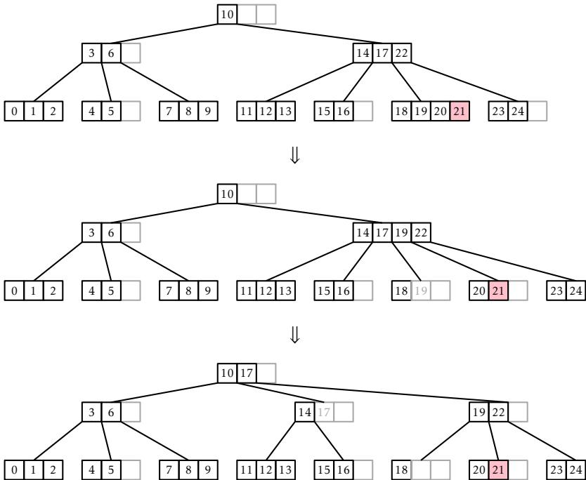
Slika 13.6: The  $\text{add}(x)$  operation in a BTree. Adding the value 21 results in two nodes being split.
