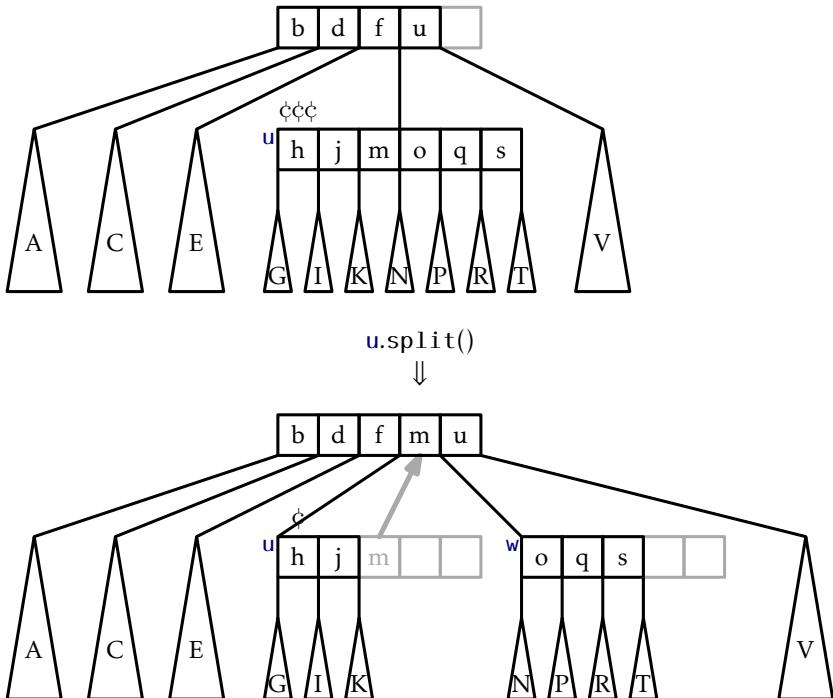
Slika 13.5: Splitting the node **u** in a *B*-tree ( $B = 3$ ). Notice that the key **u.keys[2] = m** passes from **u** to its parent.
