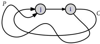
Slika 9.6: The depth-first-search algorithm can be used to detect cycles in  $G$ . The node  $j$  is coloured grey while  $i$  is still grey. This implies that there is a path,  $P$ , from  $i$  to  $j$  in the depth-first-search tree, and the edge  $(j, i)$  implies that  $P$  is also a cycle.
