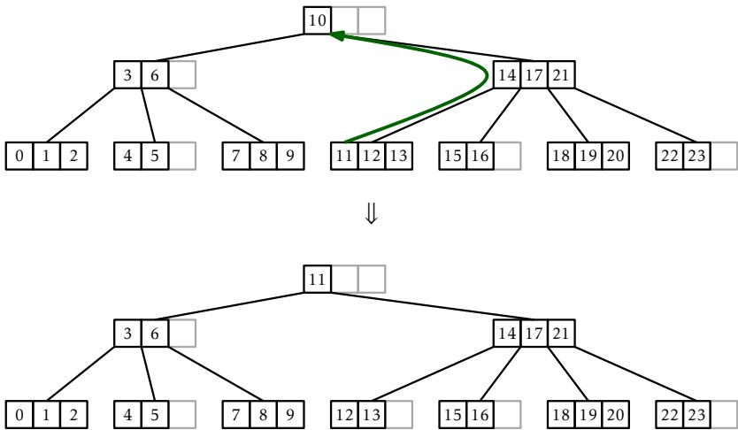
Slika 11.8: The `remove(x)` operation in a BTree. To remove the value  $x = 10$  we replace it with the the value  $x' = 11$  and remove 11 from the leaf that contains it.
