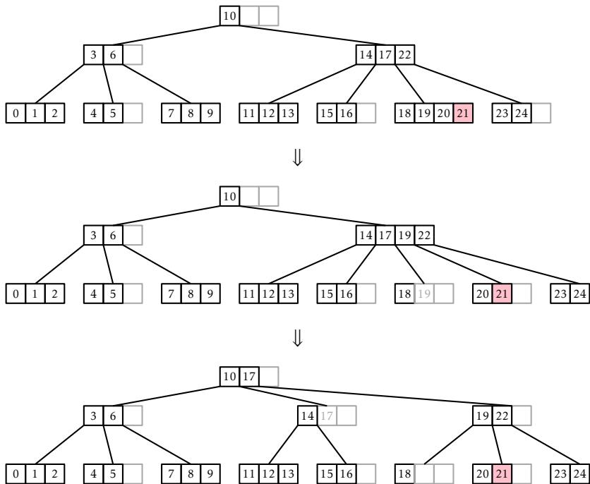
Slika 11.6: The `add(x)` operation in a BTree. Adding the value 21 results in two nodes being split.
