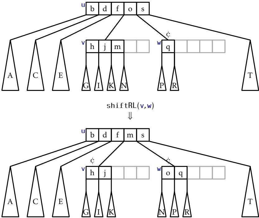
Slika 11.9: If  $v$  has more than  $B - 1$  keys, then  $w$  can borrow keys from  $v$ .
