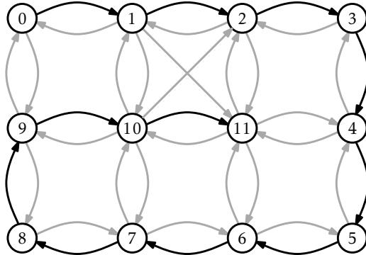
Slika 9.5: An example of depth-first-search starting at node 0. Nodes are labelled with the order in which they are processed. Edges that result in a recursive call are drawn in black, other edges are drawn in **grey**.
