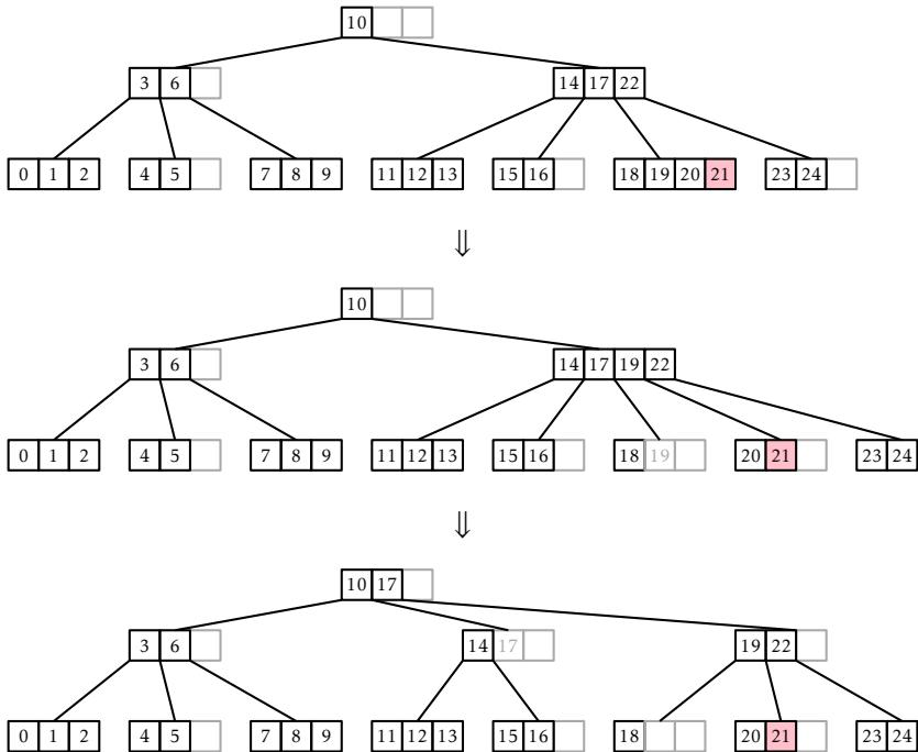
Slika 12.6: The  $\text{add}(x)$  operation in a BTree. Adding the value 21 results in two nodes being split.
