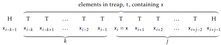
Slika 10.10: The number of elements in the treap  $t$  containing  $x$  is determined by two coin tossing experiments.
