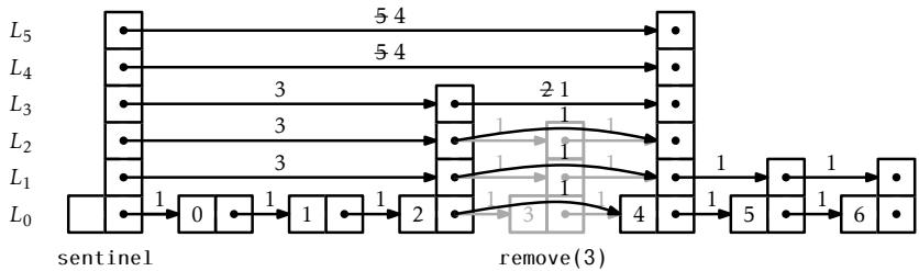
Slika 4.8: Removing an element from a Skiplist.
