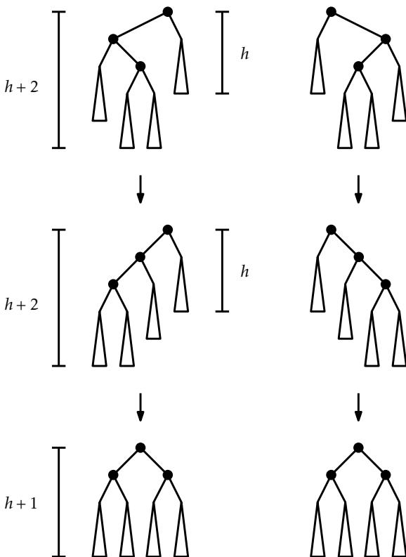
Slika 7.10: Rebalancing in an AVL tree. At most two rotations are required to convert a node whose subtrees have a height of  $h$  and  $h+2$  into a node whose subtrees each have a height of at most  $h+1$ .
