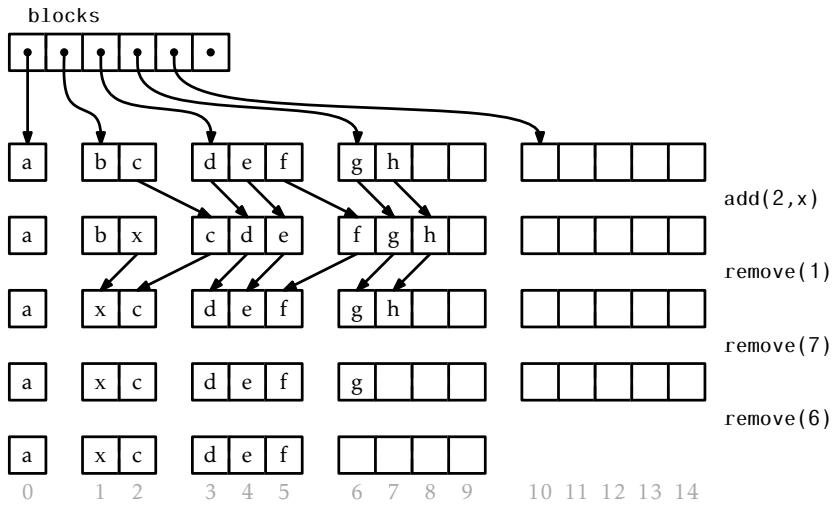
Slika 2.5: A sequence of  $\text{add}(i, x)$  and  $\text{remove}(i)$  operations on a RootishArrayStack. Arrows denote elements being copied.
